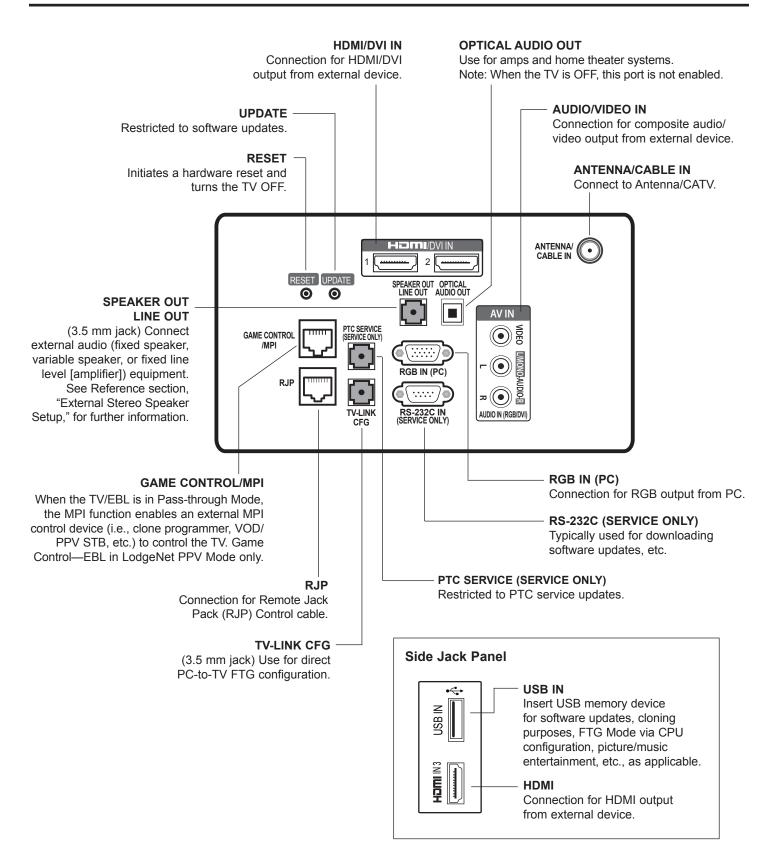
The three-contact (left, right, ground) SPEAKER OUT 3.5 mm jack on the LP645H rear panel provides stereo speaker signal outputs (fixed speaker, variable speaker, or fixed line level [amplifier]) for external audio equipment. Set Installer Menu item 097 AUDIO OUTPUT as required in accordance with external audio equipment connected to the TV. Also, refer to the following diagram for pinout details.
